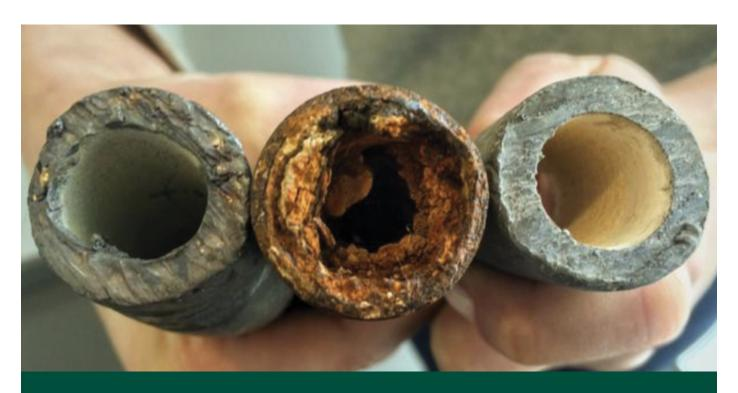
EXAMPLES (FROM LEFT) OF A LEAD PIPE, A CORRODED STEEL PIPE, AND A LEAD PIPE TREATED WITH PROTECTIVE ORTHOPHOSPHATE
